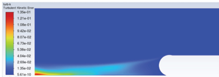
Fig. 11. Turbulence distribution at e_2/D = 0.98 , Re = 3.2 \cdot 10^5
