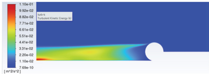
Fig. 9. Turbulence distribution at e_2/D = 0.5 ; Re = 3.2 \cdot 10^5
