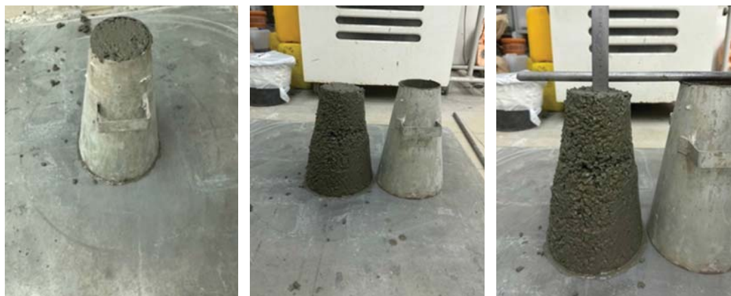
Fig. 8. Preparation of a reference concrete mix with dolomite aggregate
