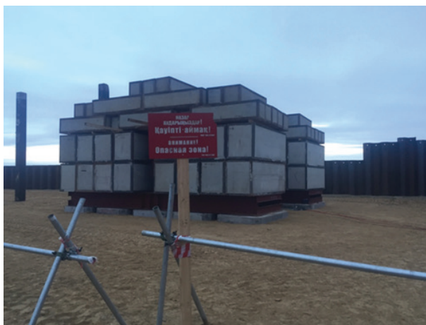
Fig. 2. SCLT static load testing of precast concrete joint piles
