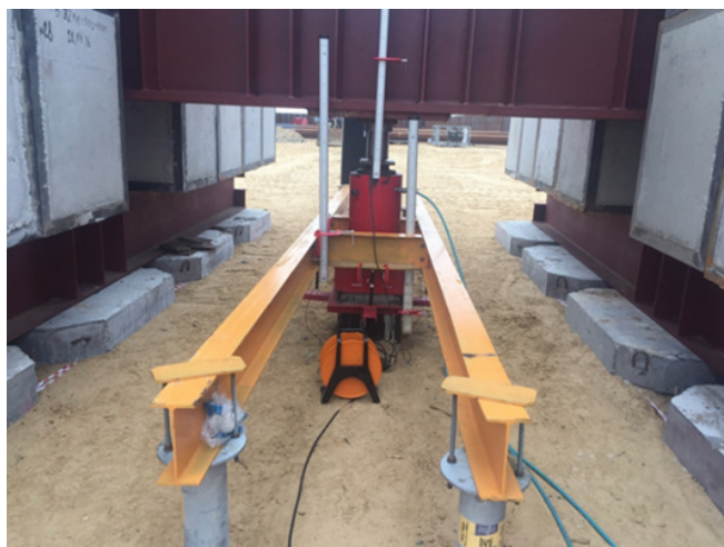
Fig. 3. Equipment for loading precast concrete joint piles
