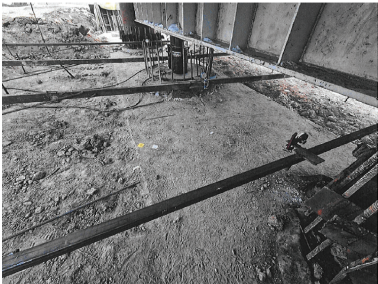
Fig. 2. System of experimental and anchor piles
