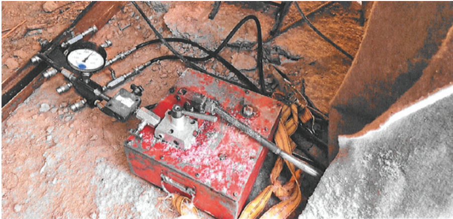
Fig. 1. Hydraulic pump with pressure gauge for pressure monitoring
