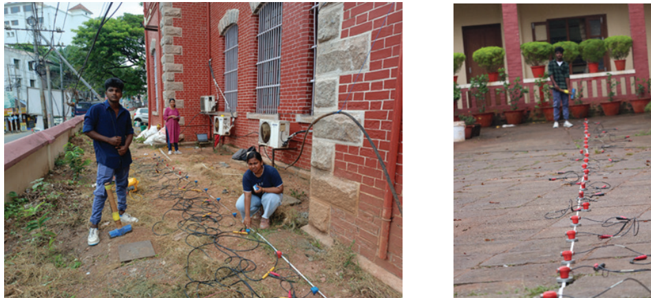
Fig. 7. MASW test setup in front and side of the PMG office building
