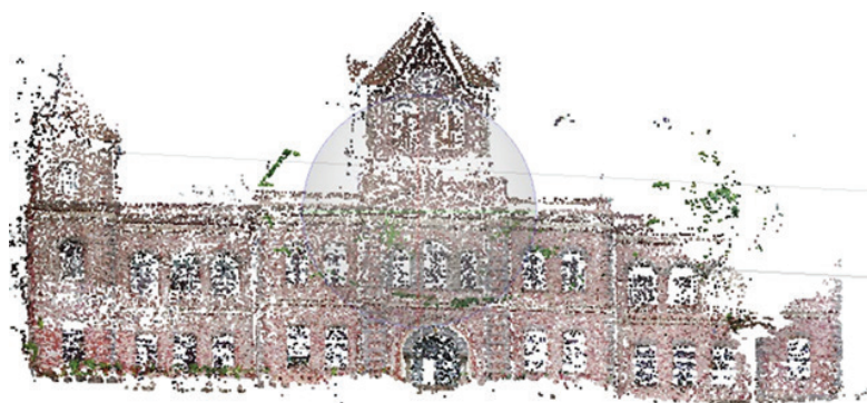
Fig. 4. Point cloud data generated after bundle adjustments
