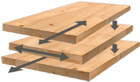
Fig. 1. Cross-gluing of CLT panels
