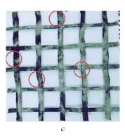
Fig. 8. Results of experimental studies of Armoset B: a — general condition of reinforced geogrid on loose sand layer; b — condition of wedging indicator (paper); c — damage of removed Armoset B geogrid
