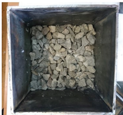
Fig. 7. Placed crushed stone layer on sand layer, paper layer and geogrid under test
