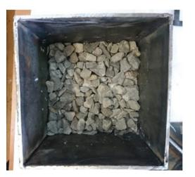
Fig. 7. Placed crushed stone layer on sand layer, paper layer and geogrid under test
