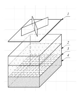
Fig. 5. Test container (metal box): 1 — metal lid; 2 — base layer (granite crushed stone M1000 fraction 20–40 mm); 3 — separating layer of geogrid and white paper sheet as an indicator to assess the jamming ability of the stone material; 4 — additional base layer — medium coarse sand
