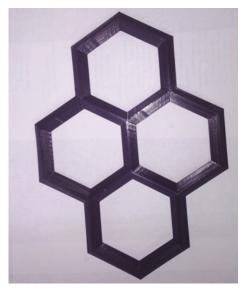
Fig. 3. Innovative 3D geogrid for pavement reinforcement
