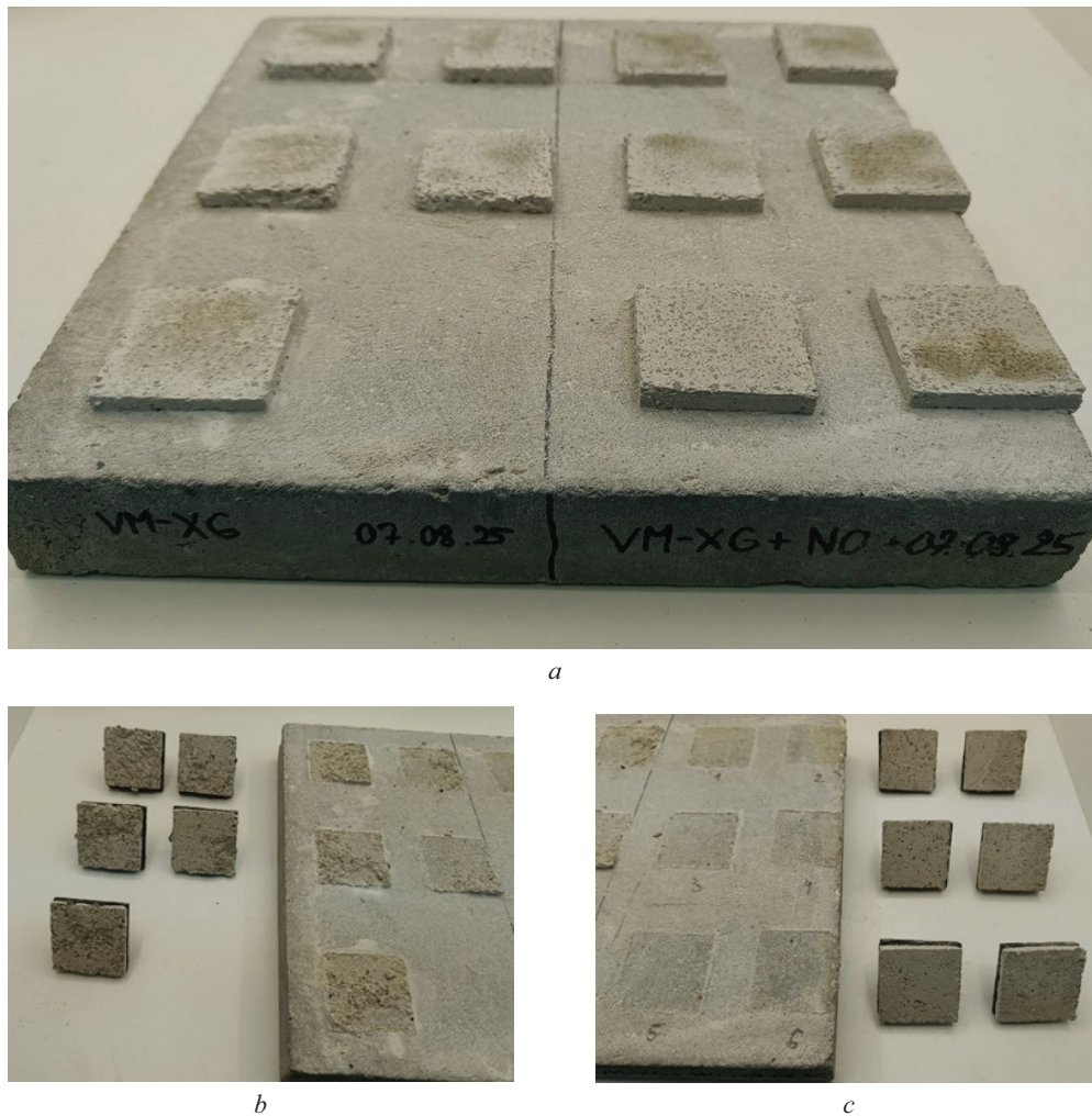
Fig. 2. Appearance of specimens for determining the adhesion strength of the material for ACP with a concrete base: a — before gluing the stamps; b — after tearing off a series of specimens with an organic modifying additive; c — after tearing off a series of specimens with an organic modifying additive and a water repellent
