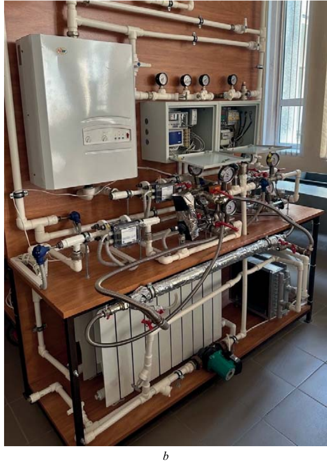
Fig. 7. Experimental setup: a — schematic diagram; b — external view; 1 — overflow; 2 — constant-level tank; 3 — mixing device; 4 — electric boiler; 5 — valve; 6 — circulation pump; 7 — valve; 8 — radiator; 9 — measuring vessel; 10 — valve; 11 — heat exchanger for primary water treatment; 12 — filter; 13 — temperature measuring device; 14 — valve
