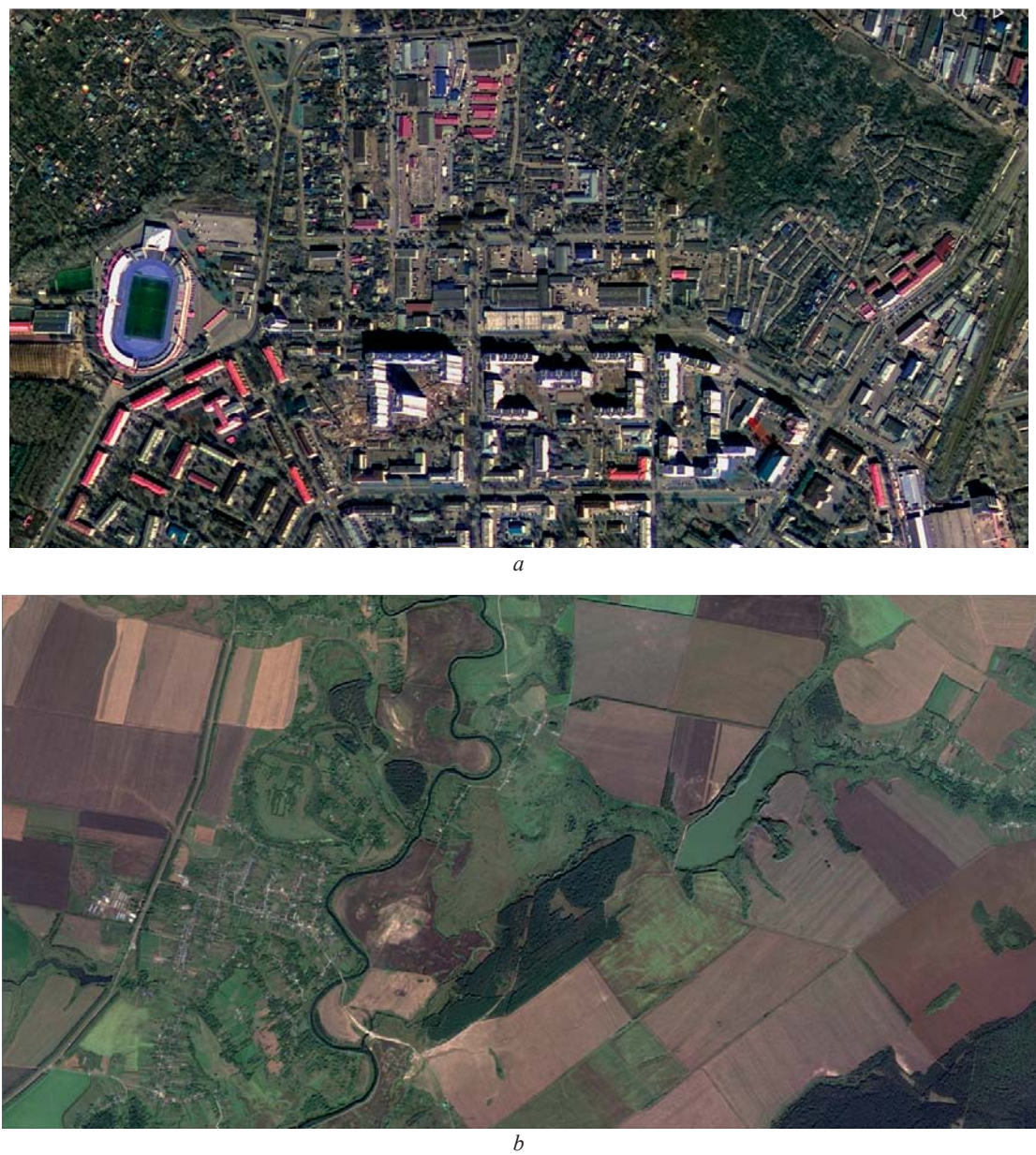
Fig. 1. Extract from a satellite image: a — Resurs-P (Russian state satellite), spatial resolution — 0.7 m; frame width — 38 km; b — Kanopus-V, ground resolution — 2.5 m
