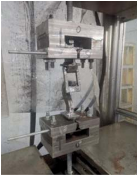
Fig. 5. Tensile test of the specimen according to X. Zou et al. [1]
