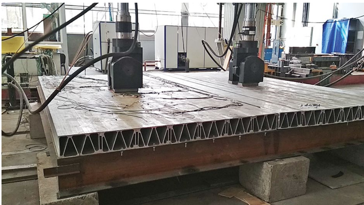
Fig. 7. Static load and fatigue resistance testing of coupled orthotropic road slabs made of EN AW-6082 T6 alloy
