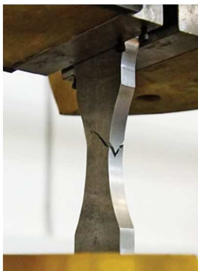
Fig. 5. View and results of fatigue tests of 1915T alloy specimens
