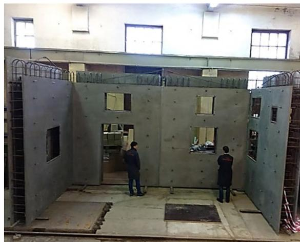
**Fig. 1.** A fragment of a room made of reinforced concrete blocks with non-removable SFRC formwork
