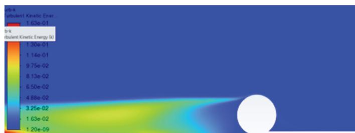
Fig. 7. Turbulence distribution at  $e_2/D = 0.1$ ;  $Re = 3.2 \cdot 10^5$
