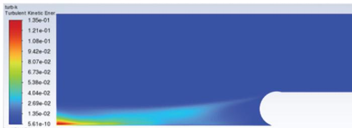
Fig. 11. Turbulence distribution at  $e_2/D = 0.98$ ,  $Re = 3.2 \cdot 10^5$
