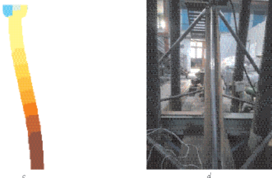
Fig. 2. Investigation of the stability of rod elements of structural coatings based on the formation of refined calculation schemes: a — finite element modelling of the nodal joint; b — “stress-strain” relationship; c — SSS picture at the loss of rod stability; d — experimental verification of the results of the numerical research (ending)
