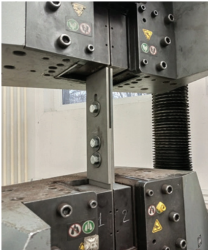
Fig. 4. Tensile testing of specimens in a tensile testing machine and scoring of steel. The width of the friction area is measured from these strongly marked areas.
