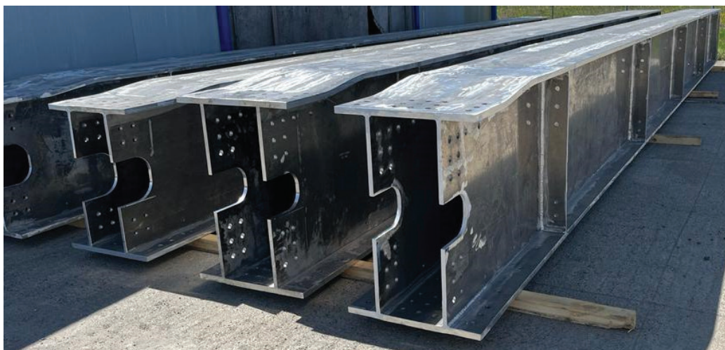
Fig. 14. Longitudinal load-bearing beams of box section
