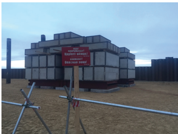
Fig. 2. SCLT static load testing of precast concrete joint piles
