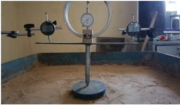
Fig. 5. Dial gauges for reading the settlement
