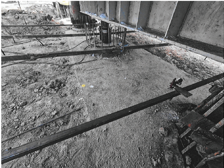
Fig. 2. System of experimental and anchor piles
