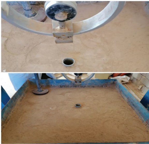
Fig. 4. Stone column inside PVC pipe
