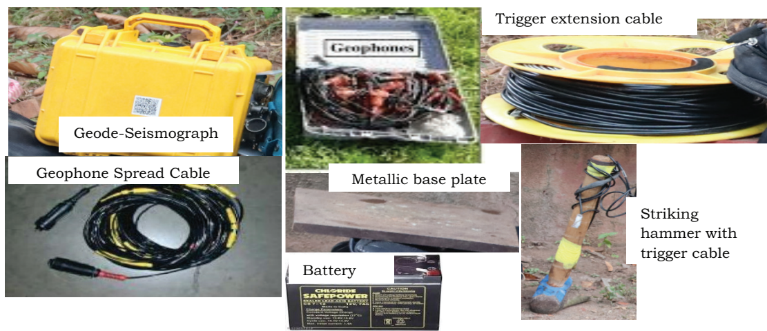
Fig. 5. MASW test setup — Equipments
