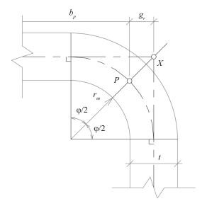
Fig. 2. Rounded corner of a thin-walled steel profile and the midpoint of the bend
