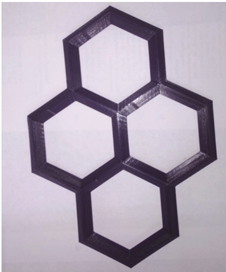
Fig. 3. Innovative 3D geogrid for pavement reinforcement
