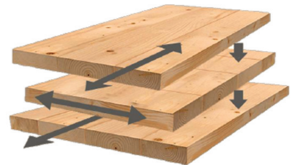
Fig. 1. Cross-gluing of CLT panels
