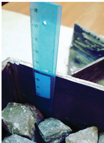
Fig. 7. Placed crushed stone layer on sand layer, paper layer and geogrid under test
