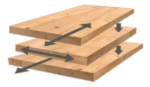
Fig. 1. Cross-gluing of CLT panels
