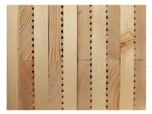
Fig. 3. The cross section of an MHM panel
