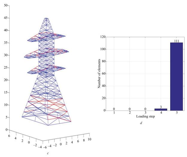
**Fig. 3.** Calculation of the U220-2+9 support (calculation situation 2): a — initial calculation diagram in MATLAB; b — 4th loading step, elements that have failed (3 pcs.); c — 5th loading step, elements that have failed (111 pcs.); d — graph of element failure during loading of the structure with a temporary load
