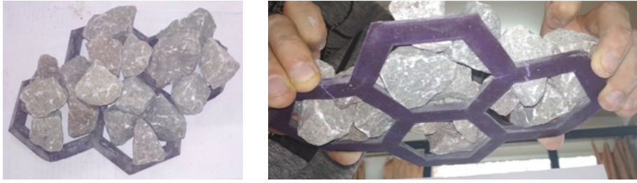
Fig. 11. Jamming of stone material in the innovative 3D geogrid
