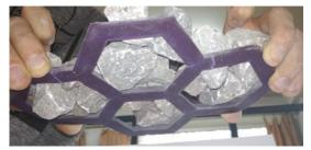
Fig. 11. Jamming of stone material in the innovative 3D geogrid
