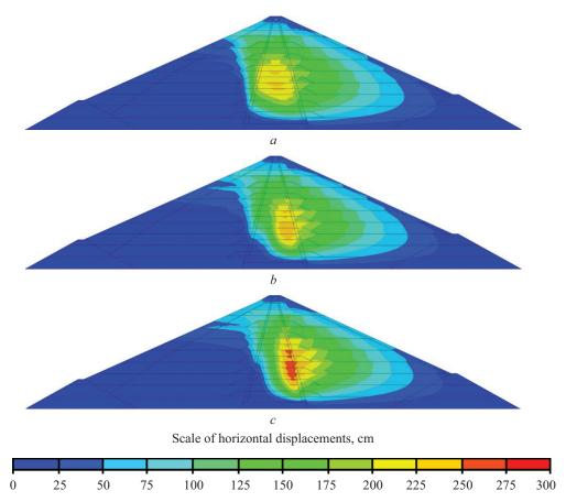
**Fig. 3.** Horizontal displacements of the dam at the end of construction for different soil permeability options: a — option No. 1; b — option No. 2; c — option No. 3
