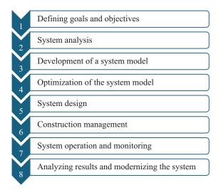
**Fig. 1.** Algorithm of working with the system within the framework of construction system engineering
