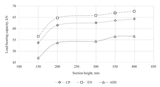
Fig. 4. Graph showing the dependence of the load-bearing capacity of a thin-walled rod on the height of the cross-section
