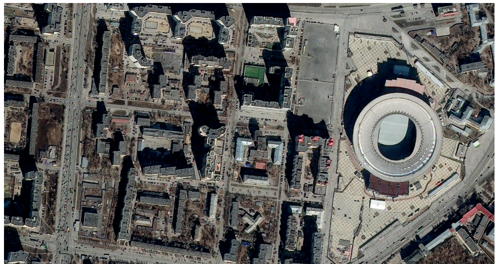
Fig. 4. A section of a Chinese Jilin-1 satellite image (EarthScanner) with a ground resolution of 0.5 m per pixel and a frame width of 150 km
